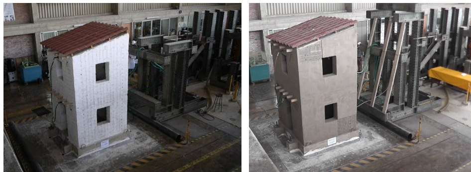
Figure 13. Panoramic view of two adobe models on the shaking table.
