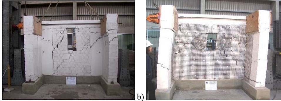
120 a) b) 121 Figure 3. Cyclin in-plane tests on adobe walls strengthened with: a) welded wire mesh and b) 122 geosynthetic mesh (Blondet et al. 2005) 123
