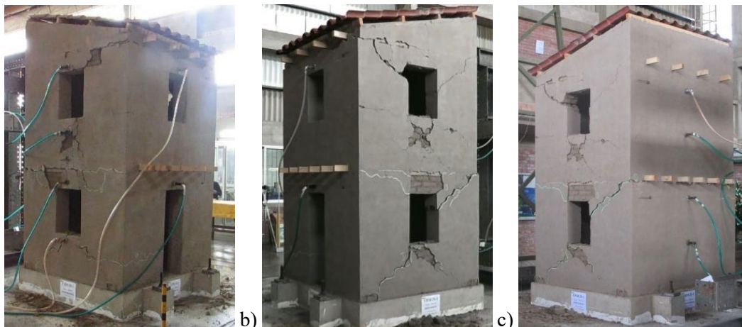
Figure 16. Adobe models after moderate shake: a), b), c) Unreinforced model; d), e) Reinforced model.
