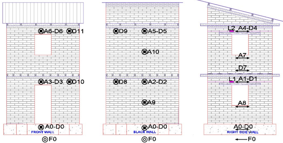
Figure 14. Distribution of LVDTs (D), accelerometers (A) and load cells (L).
