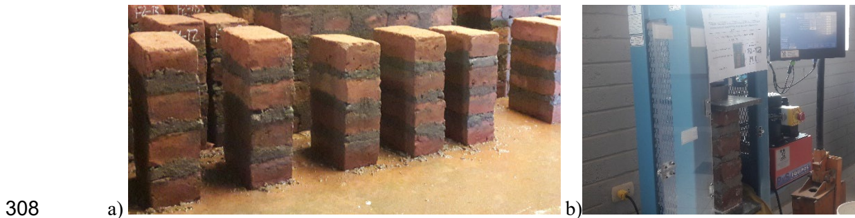
309 Figure 8. Masonry piles, a) samples, b) test set up
