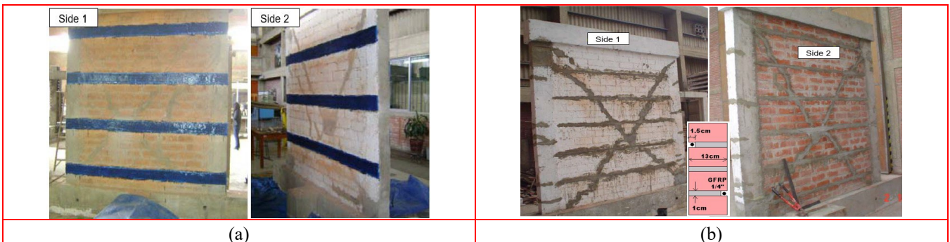
Fig. 4 FRP as reinforcement system: (a) Carbon, (b) Glass
