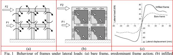
Fig. 1 Behaviour of frames under lateral loads: (a) bare frame, predominant frame action; (b) infilled frame, predominant truss action (adapted from Kaushik *et al.* 2006); (c) qualitative comparison of the experimental cyclic response of a RC frame with and without infill panels (adapted from Kakaletsis and Karayannis 2008).
