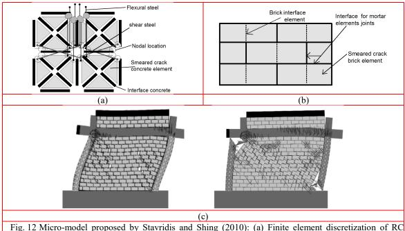
Fig. 12 Micro-model proposed by Stavridis and Shing (2010): (a) Finite element discretization of RC members; (b) finite element discretization of masonry infill (simplified micro-modelling); (c) numerical deformation and failure pattern of an infilled RC frame.
