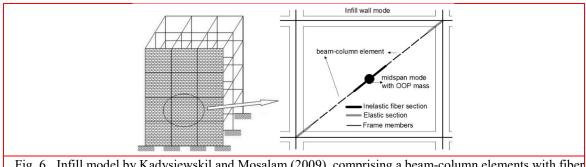
Fig. 6 Infill model by Kadysiewskil and Mosalam (2009), comprising a beam-column elements with fiber discretization (adapted from Kadysiewskil and Mosalam 2009).
