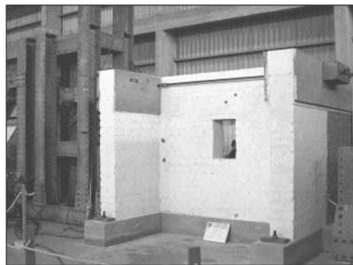
Figure 10. Adobe wall specimen subjected to cyclic lateral loading (Blondet et al. 2005).
