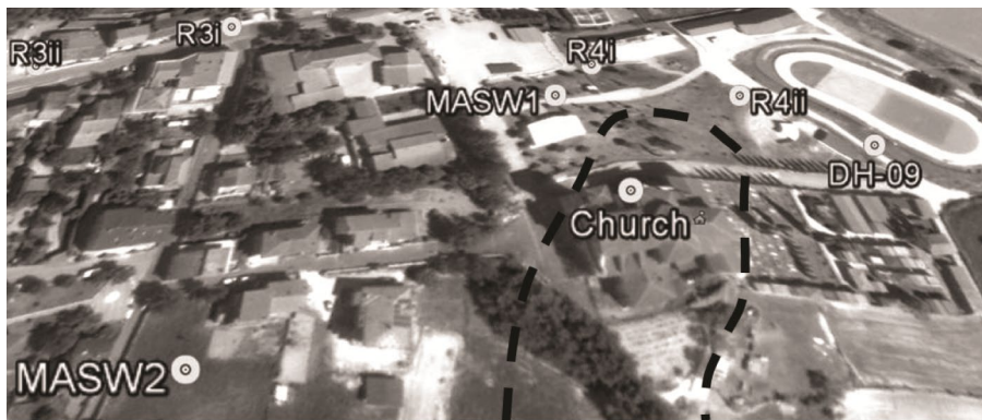
Figure 8.- Identification of additional tests performed close to the church zone. The dash line encloses the conglomerate upper layer (see Figure 5 for reference).
