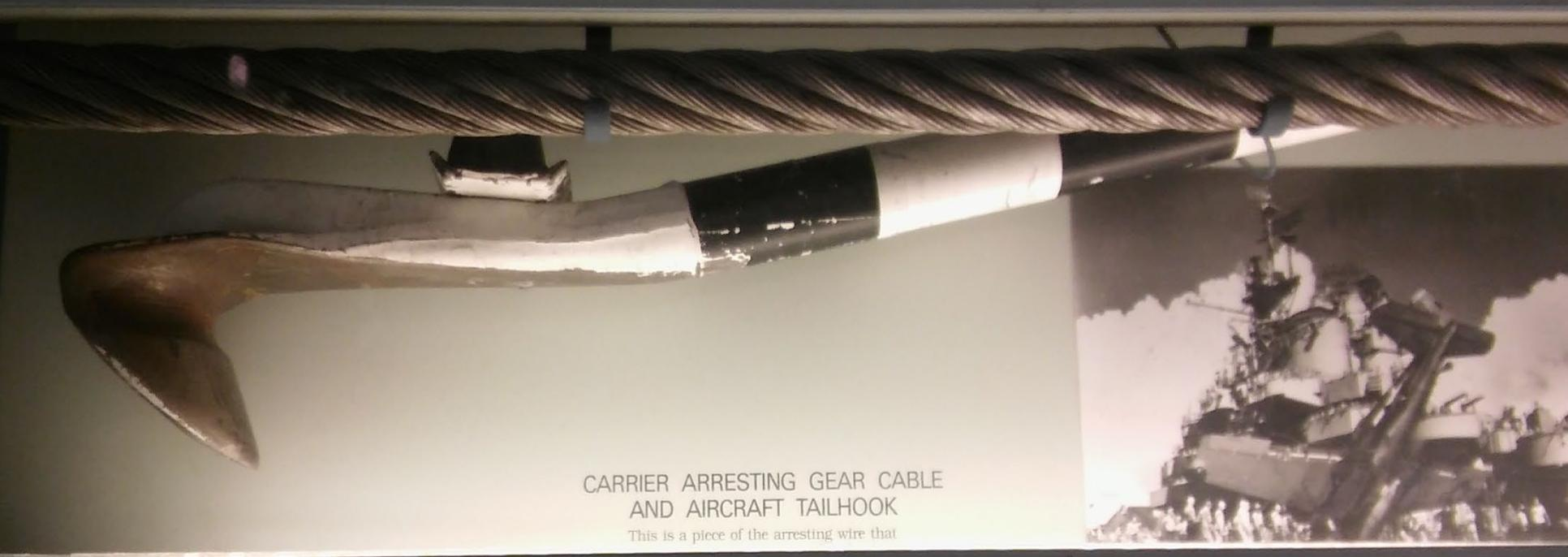
CARRIER ARRESTING GEAR CABLE AND AIRCRAFT TAILHOOK
