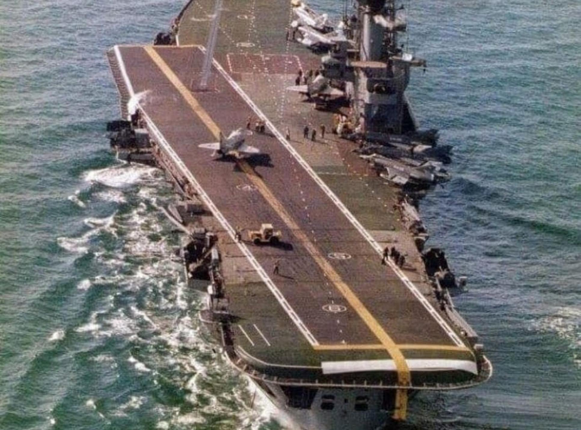
deck, with four arresting wires and a single barrier, which is rigged for emergencies only, permits the pilot to take off and fly around for another approach should he miss all of the wires with his arresting hook.
