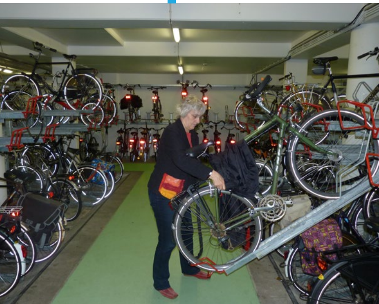
Photo 3. Two tier bicycle parking facility with integrated gas springs
