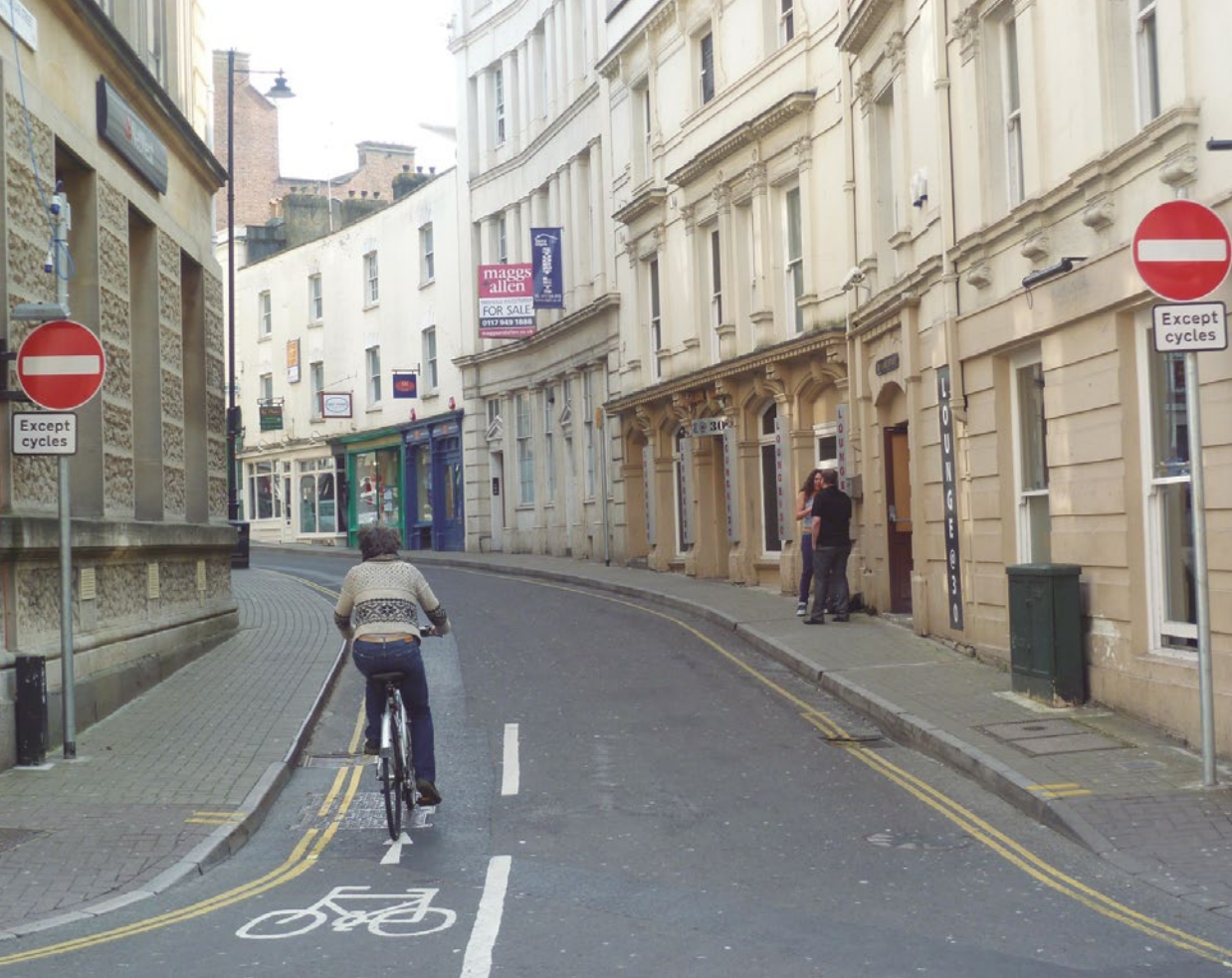
Improved permeability: contraflow cycling in a one-way street, Bristol Photo: J. Bewley / Sustrans
