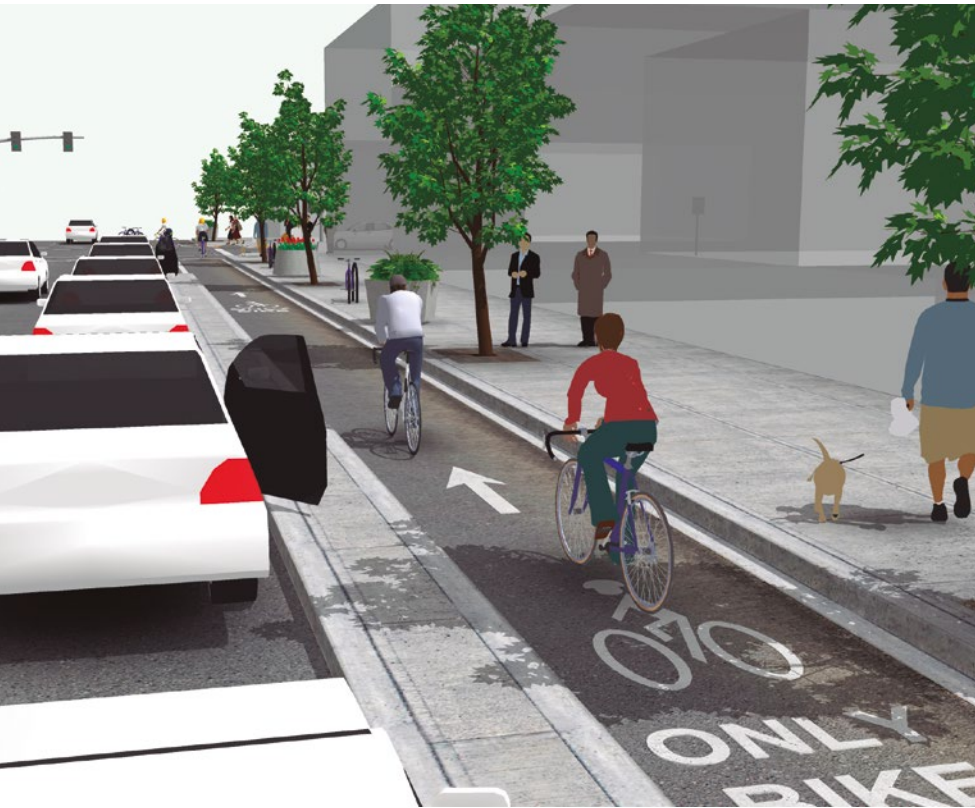
Graphic Courtesy of Alta Planning + Design One - way protected cycle track with raised curb and parking buffer. Nacto guide
