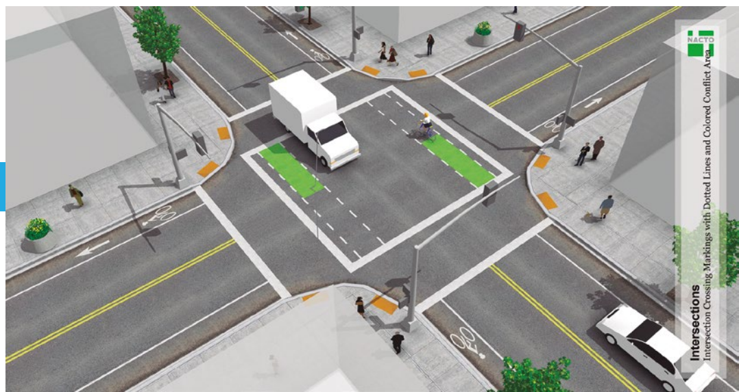
Intersection crossing markings with dotted lines and colored conflict areas. NACTO guide
