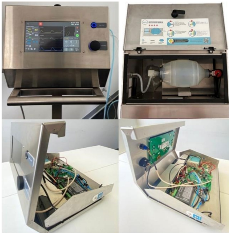
Fig. 5 Photographs of the device: a front view, b top view, c touch screen and interface buttons, d control and power boards
