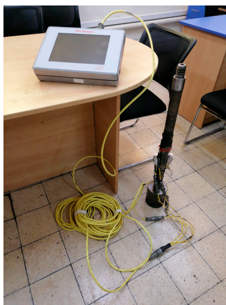
Figure 3. Pile Dynamics measurement equipment, where the accelerometers and strain gauges are directly connected to the instrumented rod section.
