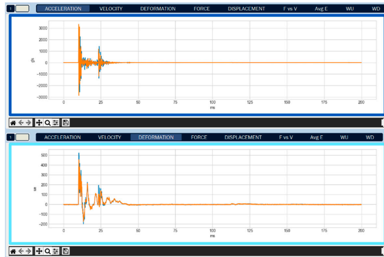
Figure 13. Visualization of two acceleration signals and to deformation signals from the test carried out at UNTELS (Kallpa Processor—Version 1.0). The graph shows two sensors per magnitude, differentiated by the orange and blue colors.
