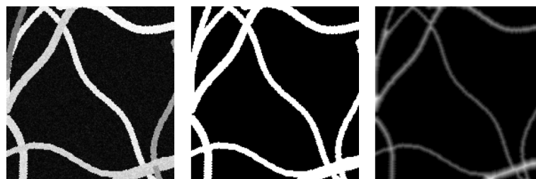
Figure 5. Distance map label steps creation: Left: source synthetic micrograph; middle: binary image from source; right: distance map obtained from binary image with Euclidean distance transform algorithm (Equation (5)).
