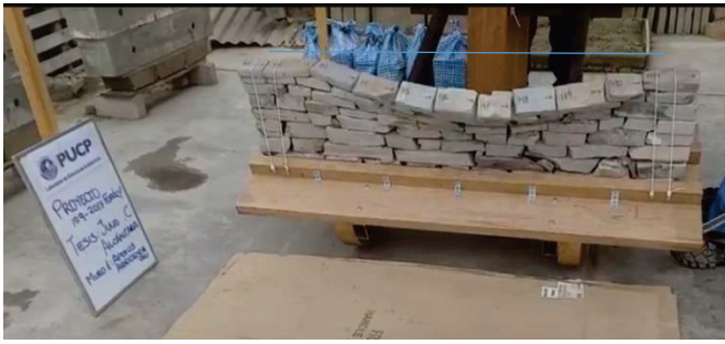
151 Figuræ7: Failure of SBR wall
