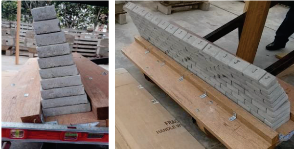
141 142 Figure 5: CBL tests (a) Relative displacement in blocks (b) Toppling failure
