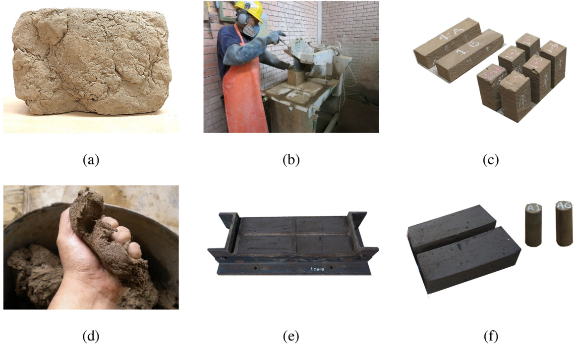
Fig. 8. Samples preparation for mechanical characterization: (a) original adobe brick; (b) sawing process of adobe bricks; (c) prismatic specimens for compression and flexure in adobe; (d) remixing process for the preparation of mortar specimens; (e) mortar on formwork; and (f) specimens for compression and flexure tests of mortar and splitting tests of adobe and mortar.
