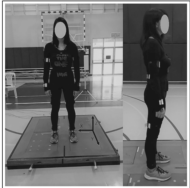
Figure 1. Inertial sensors' locations on volleyball player's body: IMU sensors on both feet, calves, thighs, arms, forearms; on both sides of the pelvis and the upper trunk; and on the forehead.
