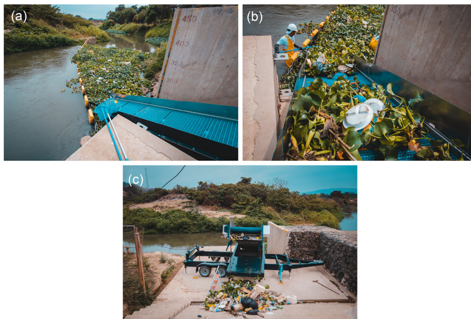
FIGURE 2 The Azure barrier system installed at the Portoviejo River, Ecuador. (a) The operating barrier; (b) operators directing litter to the conveyor belt for removal; (c) litter removed from the Portoviejo River. Source: Photos: Andrea Osorio Baquero.
