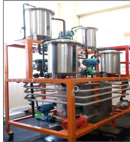
Fig. 2. Quadruple tanks process. Advanced Control Lab (PUCP)
