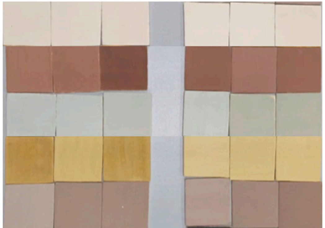
Figure 1. On the left are the paints (2, 6, 7, 11, and 12) formulated with pigments obtained through the sedimentation method (MS), and on the right are the paints (2, 6, 7, 11, and 12) obtained by the ball milling method (MG). Both have a dosage of 20%, 40%, and 60% of binder addition.
