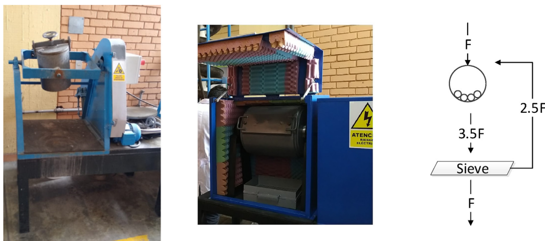
Fig. 2 – Batch ball mill (left), standard Bond ball mill (center), and Bond procedure (right).
