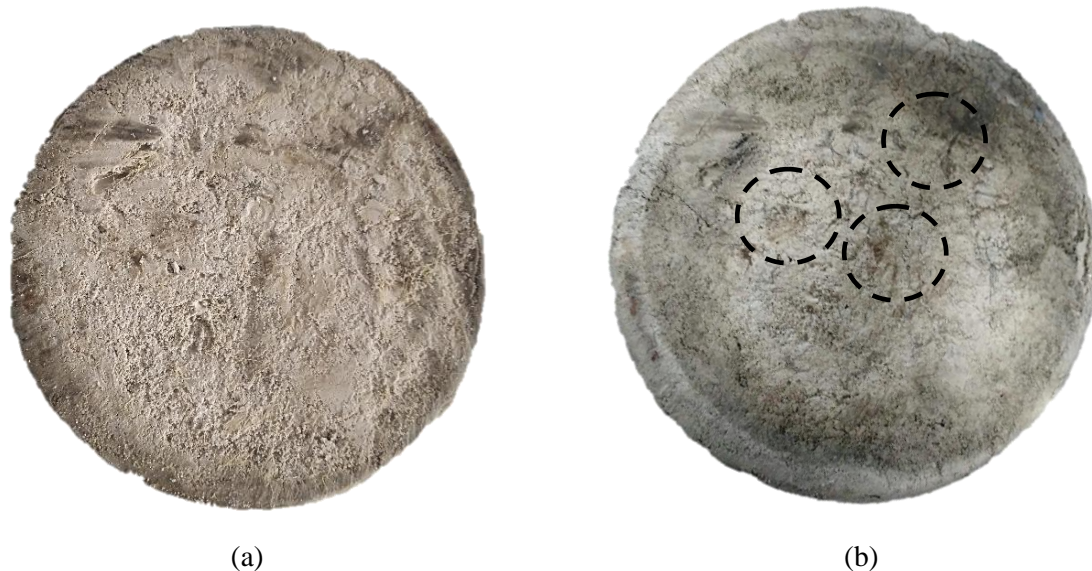
Figure 4. Fiber-reinforced lightweight geopolymer disc: (a) Before test; (b) After test.
