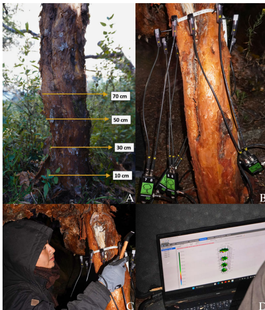
Figure 3. (A) Representation of Polylepis trunk layers. (B) Acoustic tomograph setup and sensor installation at the marked section of the trunk. (C) Measurements initiated by gently tapping the sensors with a hammer. (D) Software processes the data to identify potential areas of internal deterioration.
