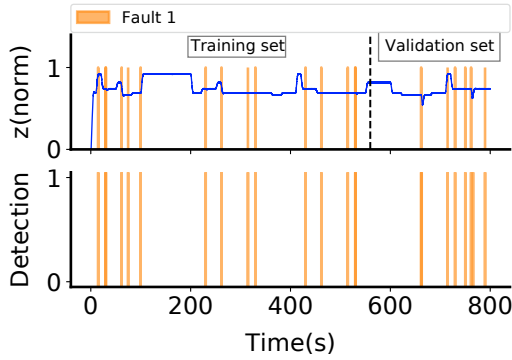
Fig. 7. Fault detection, continuous line in blue represents normalized position z , faults occurring are shown in the figure above, and detections are shown below.
